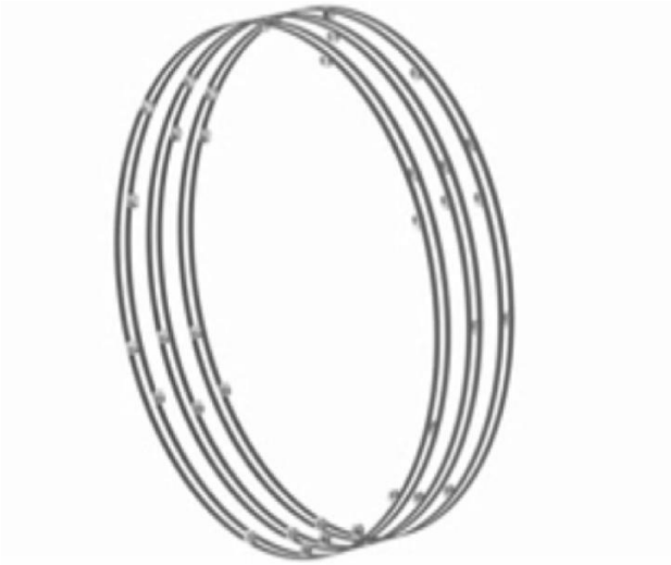
Figure 19 “Skytrak” Multi-Car Circular Transportation System operating on 360 degree tracks
